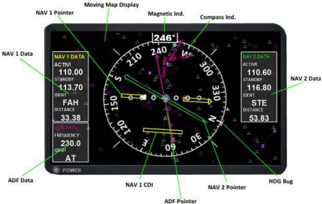
The Horizontal Situation Indicator (HSI) displays a rotating compass card with the aircraft's current heading at the top. A heading bug on the compass rose can be set to a desired heading, and the selected heading appears in a box to the left of the HSI.
