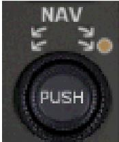
In the case of radio knobs, pressing the inner knob via right mouse click will switch control between frequency 1 and frequency 2 (NAV or COM).
