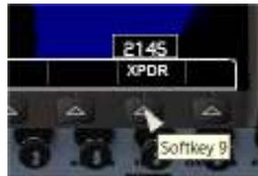
Press the softkey again and enter a code sequentially. The code is entered into the transponder automatically once the 4th digit is selected.
