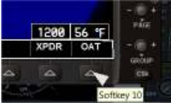
The outside air temperature is displayed in degrees Celsius at the bottom right of the MFD. Press softkey 10 to toggle the display on/off. Temperature is expressed in either Celsius or Fahrenheit depending on how the International Setting is selected in your Flight Simulator X **General Options** menu.
