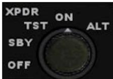
This 5-position rotary controls sets the following modes of operation, starting from counter-clockwise:
