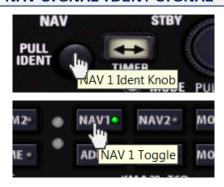
The Morse Identity signal from the Nav 1 or Nav 2 receivers can be channeled through the audio panel as follows:
